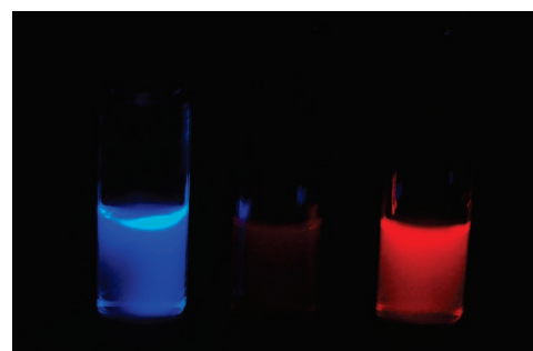
Figure 3. Emission of polymer 4 (left), 5 (middle), and 5+F - (right) in THF/ethanol (50:1 ratio) under UV irradiation (365 nm).
